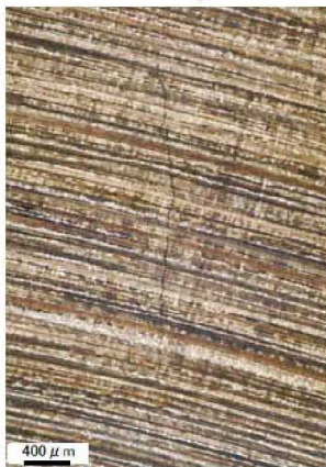
Finishing traces that are assumed to be of grinding work (polishing)
