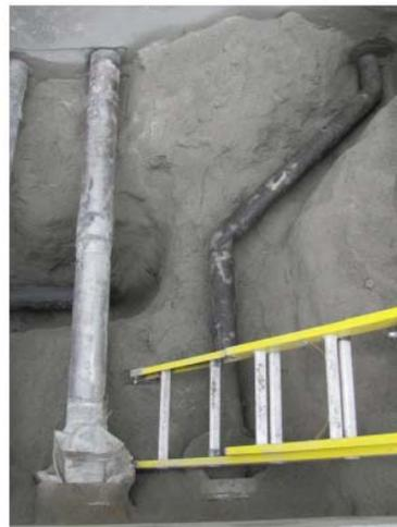
100 ft of safety-related buried pipe visually inspected with wall thickness verified by Ultrasonic Testing
